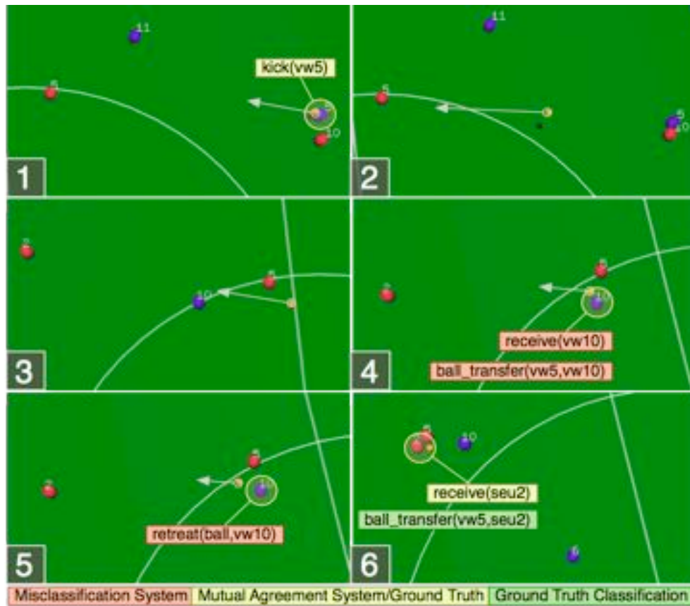
Figure 7.2: Example Situation which illustrates a premature ball transfer detection in a match Virtual Werder 3D vs. SEU
