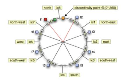
Figure 5.5: Schematic cyclic value range classification of (motion) directions with an eight-segment wind rose for a single point in time.  $ic_8$  associated with the class *north* comprises the special interval which bypasses the discontinuity point  $t_{jump}$  found at 0/360 degrees.
