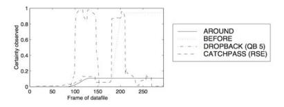
Figure 4.6: Sample likelihood curves returned visual belief networks for dropback(QB5) and catchPass(RSE) respectively superimposed with the temporal curves for dropBack(QB5) before catchPass(RSE) and dropBack(QB5) around catchPass(RSE) provided by dedicated temporal analysis functions. [IB99, p.5]
