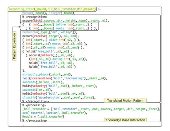
Figure 6.6: Implementation of the Prolog detection core for the *ball\_transfer* motion class. Via the *\_bound* variable and suitable additions in the motion pattern, the pattern matching process is streamlined.
