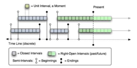
Figure 5.10: Conceptual visualization of the time model used throughout the remainder of this thesis with closed  $(I_{\parallel})$  and right-open  $(I_{\vdash})$  intervals combined.
