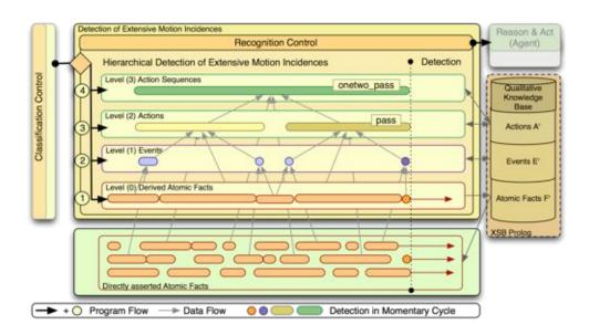
Figure 6.5: Alternative schematic overview of the course of action of a detection cycle performed by the *Recognition\_Control*. It it to show the hierarchical detection style. Starting with the assessment of new derived atomic facts the detection proceeds to extensive motion incidences thereby working towards top-level incidences. Within the same detection cycle intermediate results collected hitherto can already provide the basis for the detection of superordinate motion incidences.
